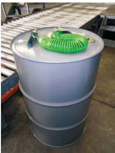
Figure 5. Typical mobile earthing for drums
